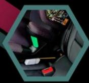
ISOFIX secures the child car seat (or seat base) to two metal anchor points built into the vehicle.
